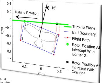
Using Monte Carlo sampling techniques, we simulate a large number (>1 million) of flight paths to estimate the mean collision probability of individual birds. This is then used in conjunction with observed passage rates to estimate the annual risk of collision.
